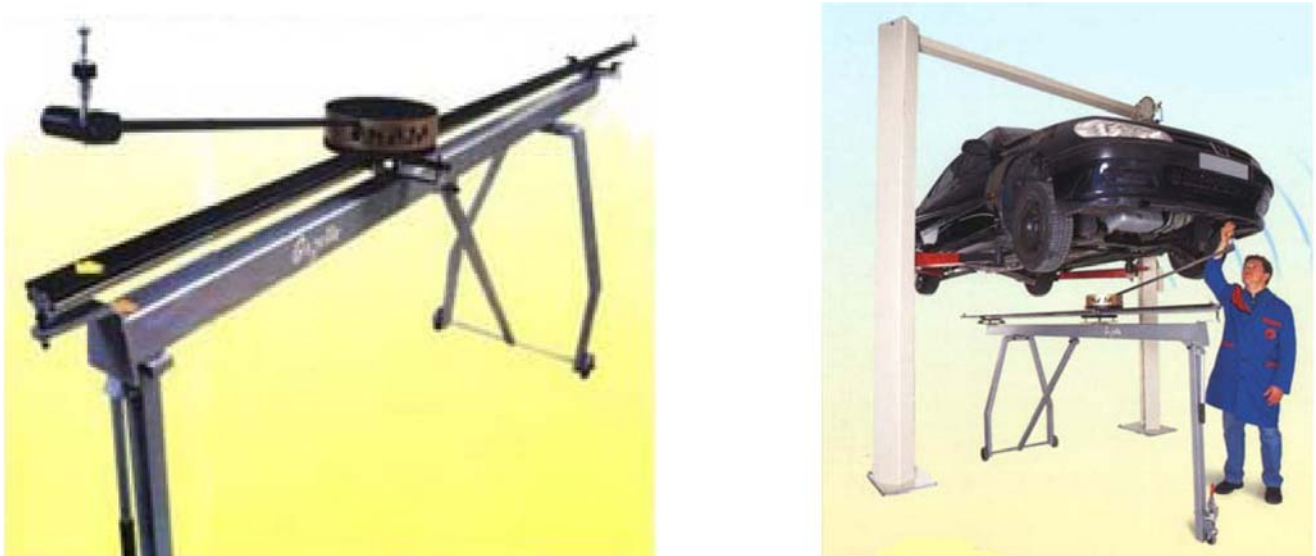
Fig. 8. The NAJA measuring system and an example of using
