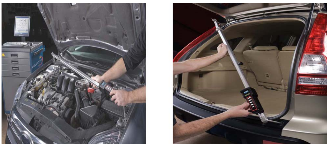
Fig. 4. Examples of measurements with the use of Intelli-Tape
