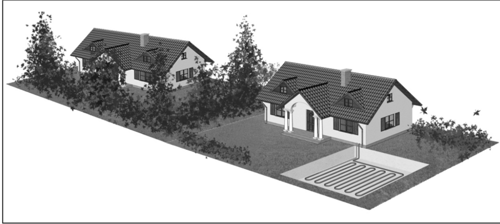
Fig. 1. Heat pump with a horizontal installation and reduction of number of trees (author's own study)
