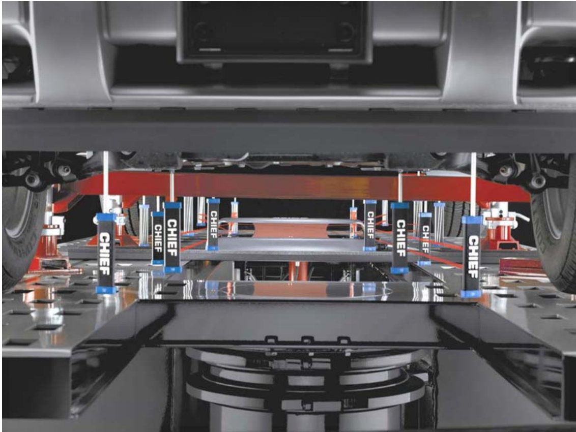
Fig. 7. Positioning of measuring heads and scanning laser during floor plate measurements
