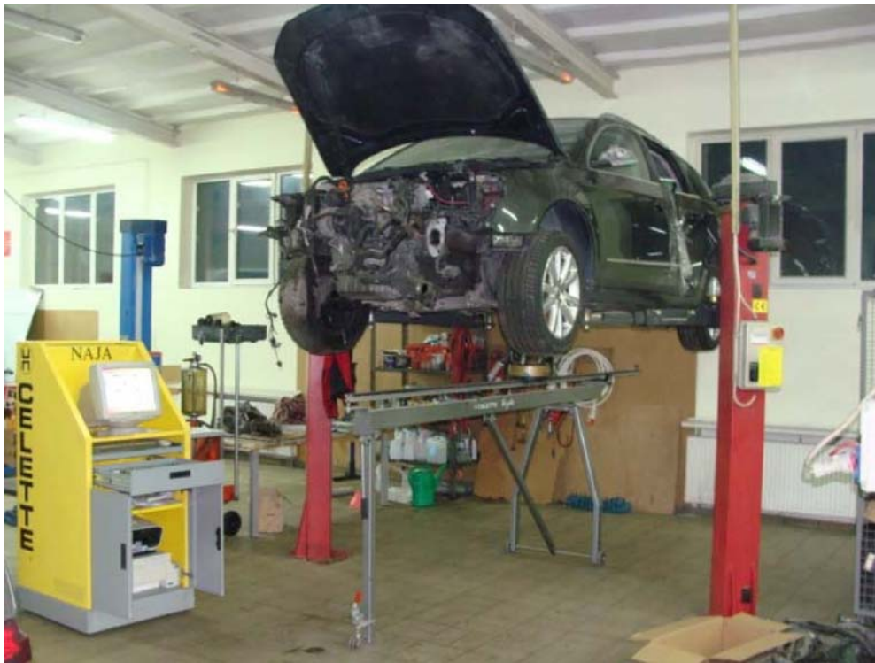
Fig. 9. The investigation of VW Passat car body with the use of NAJA measuring system
