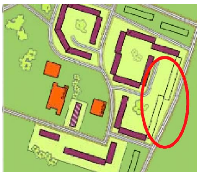
Fig. 6. Destroyed buildings as acoustic screens on edge of housing area
