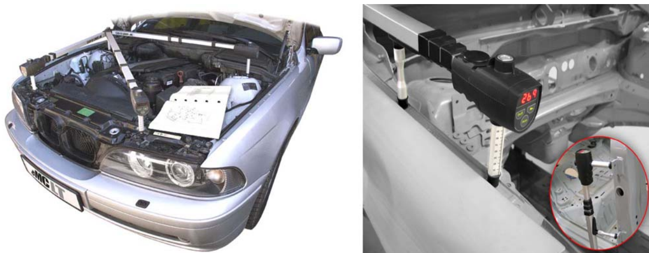
Fig. 3. Examples of measurements with the use of eMC LT system
