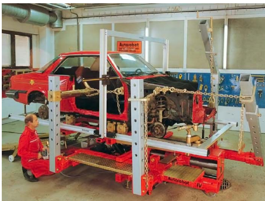
Fig. 10. The view of the Autorobot repairing device with measuring system and repaired vehicle
